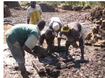
Making mud bricks Malawi style
